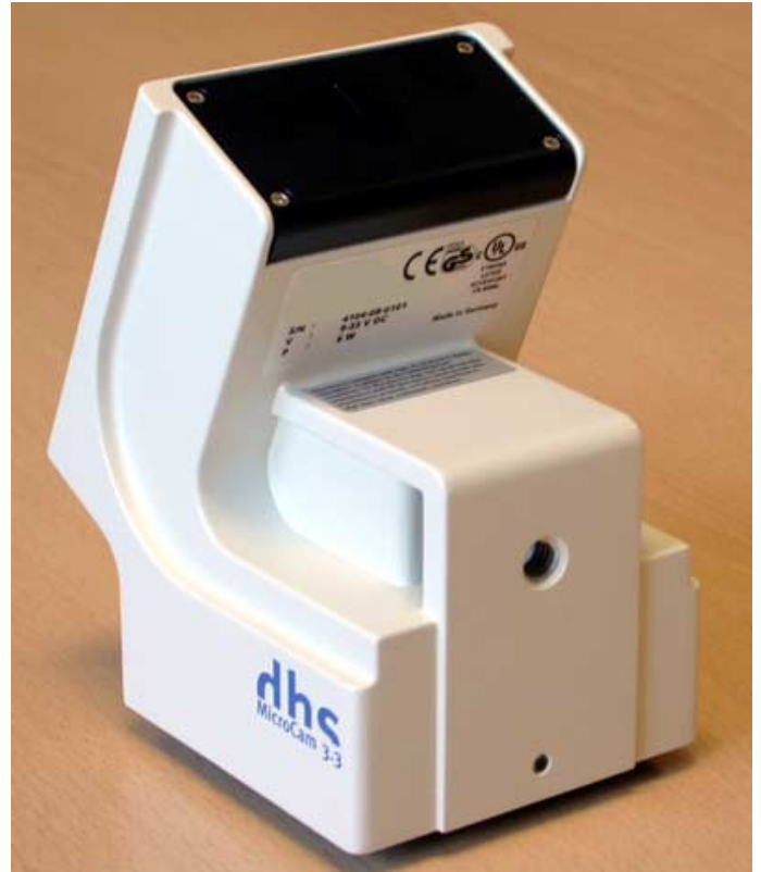
Rear view of the camera with FireWire port and socket for macro copy stand
