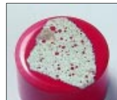
EPO-COLOR™ appears bright red under darkfield or polarized light
