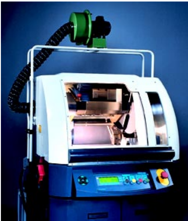
The 10-2342 Fume Extractor filters and reduces emissions.
