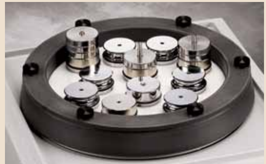
Generous specimen capacity allows up to 18 specimens to be prepared simultaneously.
