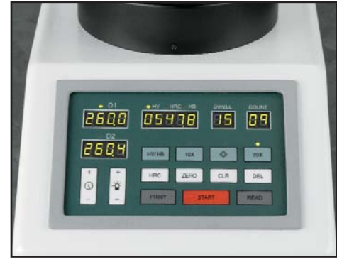
Left). The IndentafMet 1106 has a motorized D1/D2 prism photo port and turret. All models have an indenter protector sleeve to reduce the chance of accidental indenter damage. Middle). IndentafMet Testers have easy-to-use digital touch pad controls that shows all vital information including D1 and D2 diagonal lengths, Hardness scale and value, dwell time, count, and objective. Right). The IndentafMet Macro and Semi-Macro Vickers Testers touch panels have load, D1 & D2 diagonal length, hardness value and converted value.
