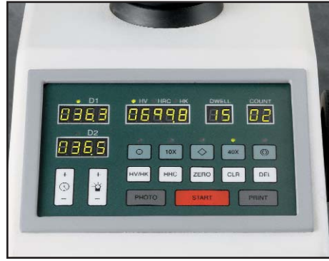
Left). The IndentafMet 1106 has a motorized D1/D2 prism photo port and turret. All models have an indenter protector sleeve to reduce the chance of accidental indenter damage. Middle). IndentafMet Testers have easy-to-use digital touch pad controls that shows all vital information including D1 and D2 diagonal lengths, Hardness scale and value, dwell time, count, and objective. Right). The IndentafMet Macro and Semi-Macro Vickers Testers touch panels have load, D1 & D2 diagonal length, hardness value and converted value.
