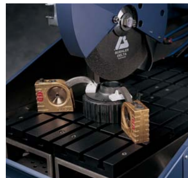
10-3523 Irregular specimen vises secure unusual sample sizes.
