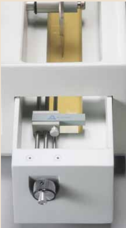
Dressing chuck is conveniently located within the coolant tray.
