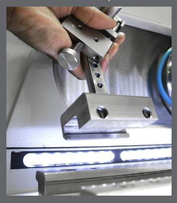
Buehler's Rapid Rail System allows for users to secure samples in the cutting chamber and begin the next cut within seconds.
