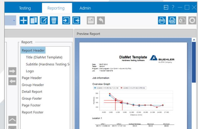
Verify the readings in graph grid and remeasure or re-indent where applicable. Export results to a PDF, a printer or in Excel®.
