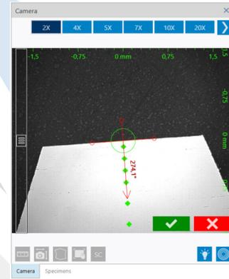
Use the overview camera or infinite scan to see where all indents will be placed. Press **start** to indent and measure all.
