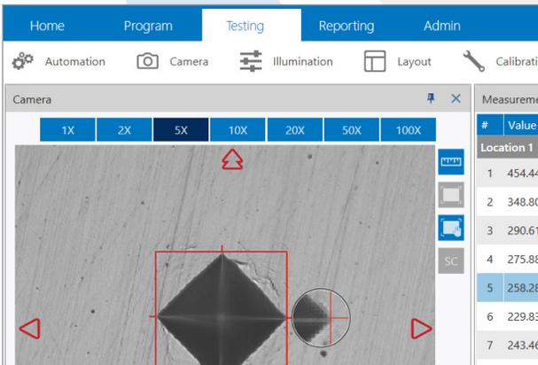
Machine and software make all indentations and measure them automatically, using the standard\* automatic focus, illumination and measurement functions.
