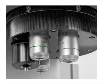
The precision mechanics of the motorized turret, allows for a fast and quiet positioning. Switching between indenter and objective is part of the automated test cycle.
